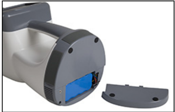
Figure 2-2 Battery chamber with the cover removed
