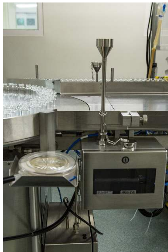
Figure 1. Viable and nonviable sampling points (BioCapt® Single-Use and Airnet® II Particle Sensor)
