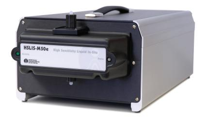
The HSLIS e-Series (High Sensitivity Liquid In Situ) particle counter provides continuous, real-time monitoring of contamination levels in DI water and process chemicals. The combination of high sensitivity and low cost makes it ideal when large numbers of sensors and/or long term trending are required.
